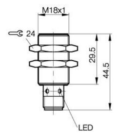
**Inductive Sensors** BES 516-367-E5-Y-S 4 M18x1 x 44.5 normally-closed Sn=5mm shielded
